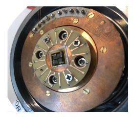
Here, a new class of planar waveguide devices are shown, that elucidate the exciting physics that can be explored and the pormising quantum-photonic applications that can be developed with such on-chip dipolariton circuits: we demonstrate that remarkably, "dipolar light" can very effectively undergo coherent scattering from local electrical potentials, in a manner consistent with quantum scattering theory of ultra-light dipolar particles.
